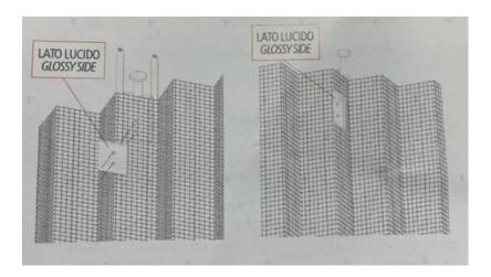
• Before you replace the mesh insert the slider into the top track. You can use the screw driver to assist with positioning the insert. See drawings below.
