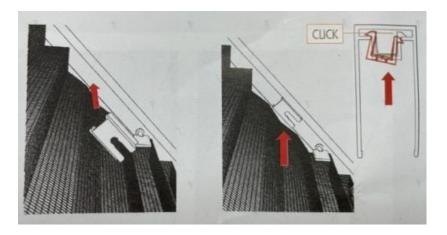
• Push the mesh back into the top track and slide the protrusion on the clip into the slider until it clicks. See images below.
